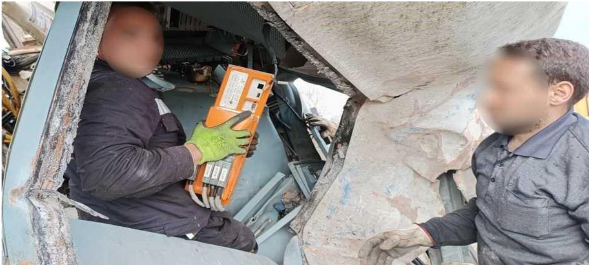
Figure 54. On board TELOC data recorder, train 63503, locomotive 120-022, retrieved by judicial experts on the 05.03.2023.
