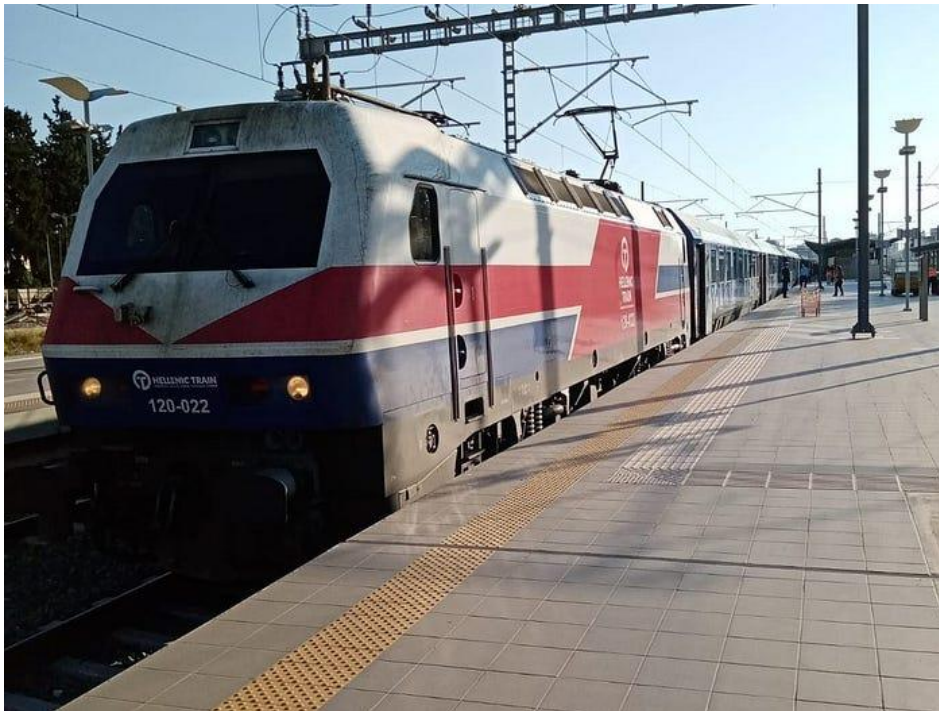
Figure 69. First locomotive, Siemens Hellas Sprinter 120-022. NVR Engine: 91 73 212 0 022-7. Last maintenance "I1" 23/02/2023, Thessaloniki.
