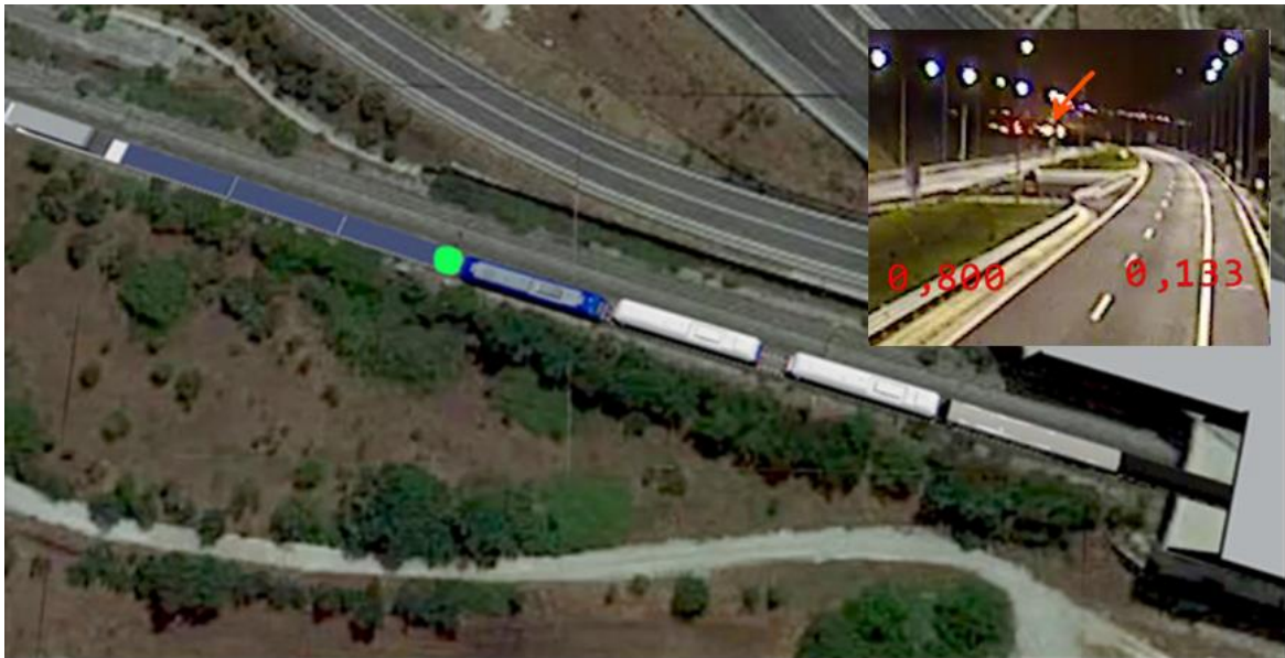
Figure 18. Estimated area for second collision for the freight train (simulated image behind still of video footage).
