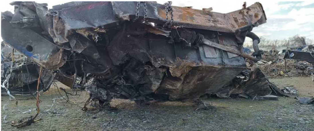
Figure 85. Position 1) 120 023 locomotive, totally destroyed, broken into large pieces. Remaining piece of the basement platform. Part with transformer still visible. Other side in Figure 17. At the position 2) the A1 1st class coach, totally destroyed, has broken into small pieces, and was not recognisable as a whole vehicle.
