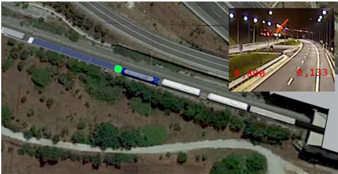
Figure 58. Estimated point of initial ignition.
